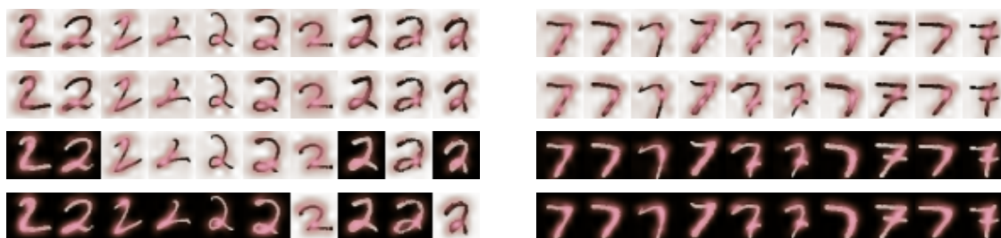
Figure 1: Explainable classification with Grad-CAM: training iteration 0, 1, 10 and 50 (from top to bottom). The color intensity corresponds to the value of gradient-weighted class activation mapping. The white background images are misclassified, the black ones are classified correctly.
